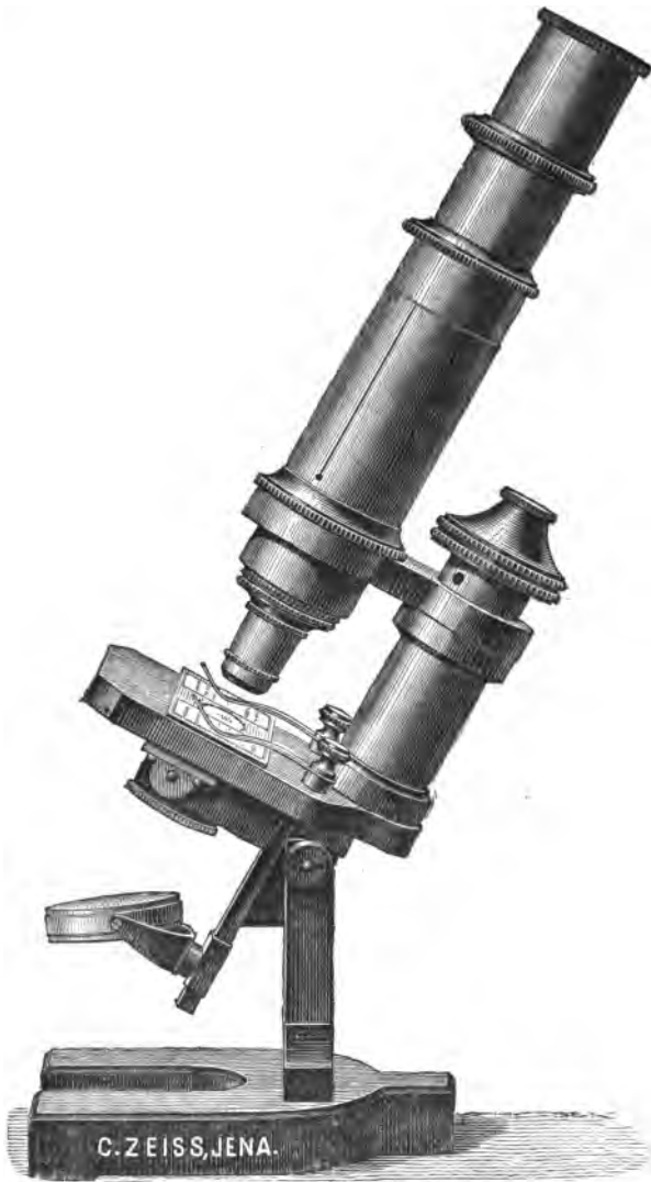
FIG. 8.—Zeiss's Stand VI., provided with a hinged stand, a draw-tube, cylinder diaphragm, and mirror with a concave and a flat surface.
